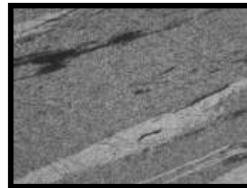
Fig.9. Stirring zone in 2-path stirring workpiece
