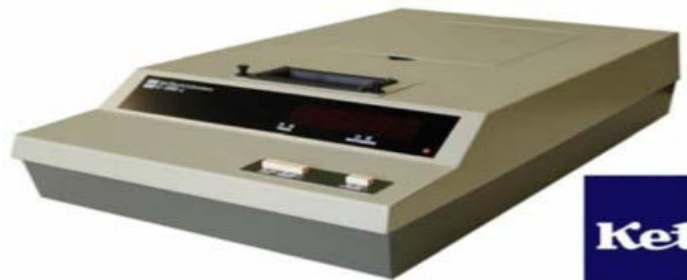
Fig. (4): The grain whiteness meter
