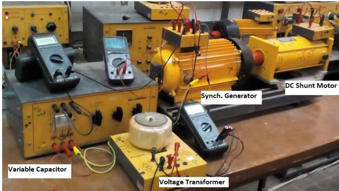
Figure 4- Photo of the experimental setup of the SPSESG.
