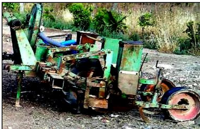
Fig. 1: Soffgia precision vacuum planter
