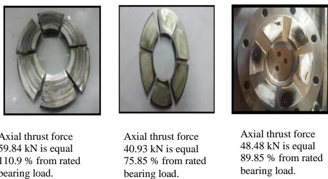
Fig. 13: Axial Thrust Force Effect on Thrust Bearing
