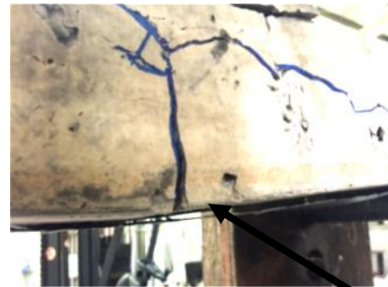
c) Numerical and Experimental failure mode of medium reinforcement ratio with 2 Layer
