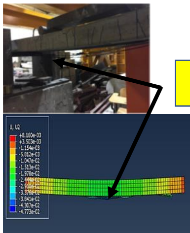
b) Numerical and Experimental failure mode Of medium reinforcement ratio with 1 Layer
