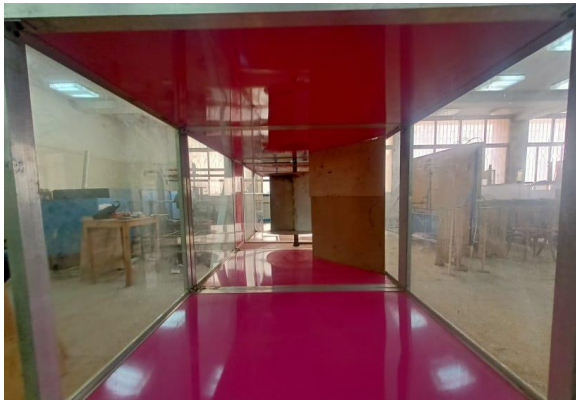
Fig. 4. A photograph for the test rig of the Savonius rotor inside duct with obstacle plate
