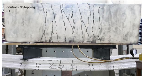
Fig.12: Crack patterns, crack distribution and failure mode for control specimen C1
