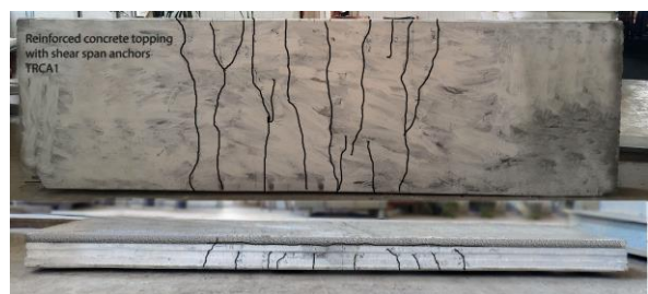
Fig.14: Crack patterns, crack distribution and failure mode for specimen TRCA1
