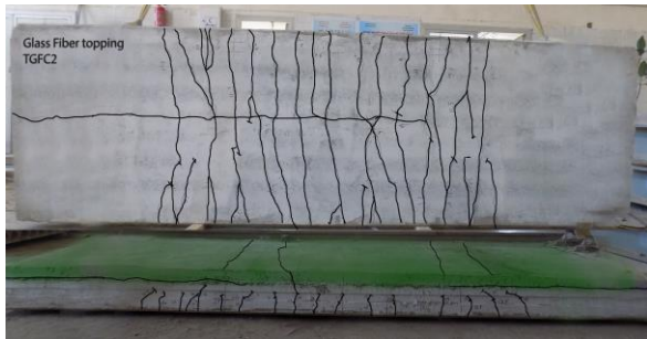
Fig.17: Crack patterns, crack distribution and failure mode for specimen TGFC2
