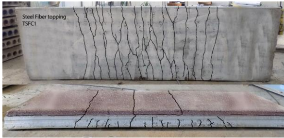
Fig.16: Crack patterns, crack distribution and failure mode for specimen TSFC1
