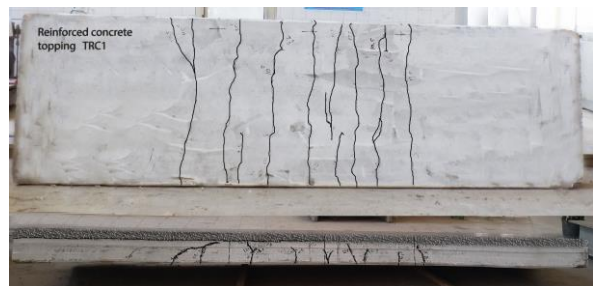
Fig.13: Crack patterns, crack distribution and failure mode for specimen TRC1
