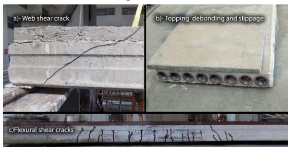
Fig. 19: Some cracks modes and slippage of concrete toppings in tested specimens
