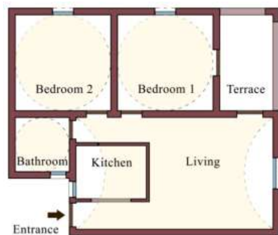
Fig. 4; Architectural design of typical unit
